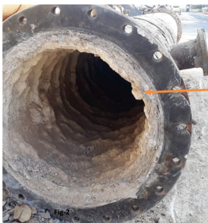
Figure 1. Scaling inside a MSRL pipe.
