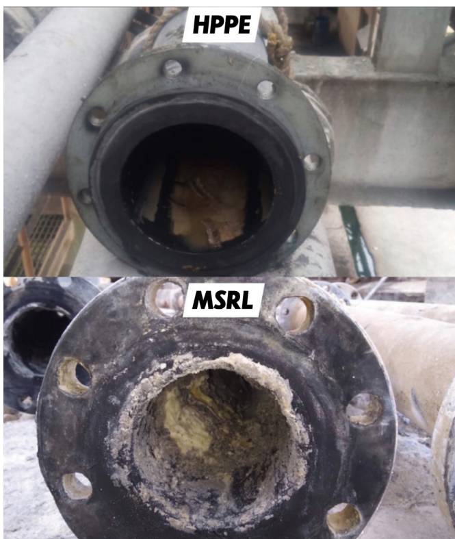
Figure 3. Scaling comparison between HPPE and MSRL pipe.
